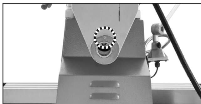
Figure 64. Horizontal spindle arbor support ball oiler.
